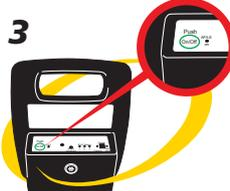
Press the amplifier's on/off button once - the amplifier will beep to confirm it is ready to use.
