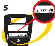
Check the amplifier's 'AFILS working' indicators to ensure they illuminate in line with your speech (1 & 2 is normal, 2 & 3 is too loud).
